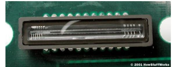
A Scanner's CCD Sensor
